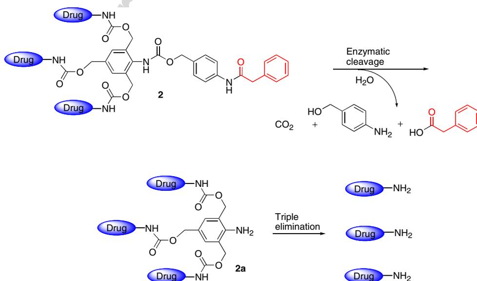
Figure 2. Disassembly mechanism of AB<sub>3</sub> self-immolative dendritic molecule **2**.
